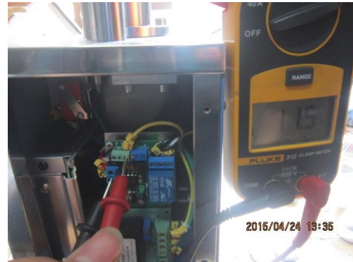
Adjust Sampling voltage (8 - 12V)
